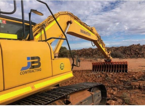
**Excavator with 3m scarifier for site scarification & vegetation spreading.**
