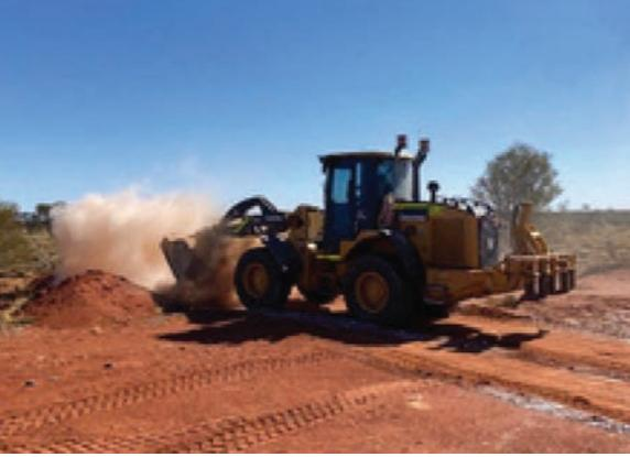
**Loaders with custom built frontmount scarifier & rear rippers.**
